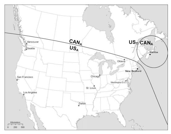
Fig. 4. Isolines defining the locations where energy costs are equivalent for the paired comparisons of air freighted Canadian Atlantic scallops to those truck or air freighted from the US. CAN scallops can be truck freighted to New Bedford for less energy than that needed to produce scallops there, and thus there is no CAN<sub>T</sub> isoline.
