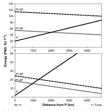
**Fig. 3.** The  $E_{P\otimes D}$  for seafood products produced in two locations 4800 km apart. The product from *P* is distributed by air, while *P'* is distributed by truck. *P'* is two (thin dotted line) and five times (thick dotted line) as costly as *P*, respectively, where  $P = 2 \text{ GJ} \text{ T}^{-1}$  (bottom) and 20 GJ T<sup>-1</sup> (top). As the base cost of production increases, the implication of the alternate source having a relative larger production cost is much greater.
