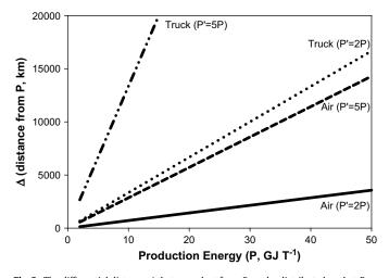
**Fig. 2.** The differential distance  $\Delta$  that a product from *P* can be distributed so that  $E_{P&D}$  of P = P'. The value of *P* is on the *x* axis, and *P'* is 2 or 5 times larger.  $\Delta$  increases as the cost of production increases, as the relative value of *P'* increases with respect to *P*, increases more rapidly when the product is distributed by truck as compared to air. As a reference, the distance from New Bedford MA to Seattle WA is approximately 4800 km.
